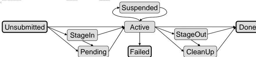
Figure 8: State transition diagram for GRAM jobs.
