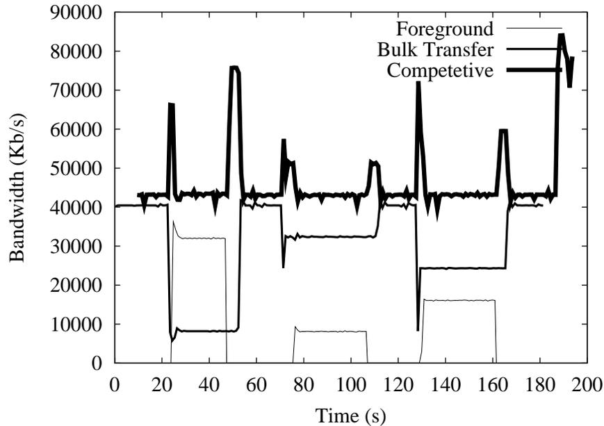
Figure 5. Performance achieved for a mixture of Premium and Best-Effort services on GARNET. We demonstrate that a bulk-transfer (background) application is able to exploit unused Premium traffic without affecting foreground reservations. See text for details.
