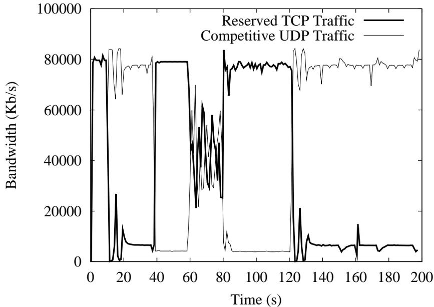
Figure 11. Performance achieved for a TCP flow in the presence of competing UDP traffic and host load, for various combinations of network and CPU reservation. We demonstrate GARA’s ability to co-reserve multiple resource types.
