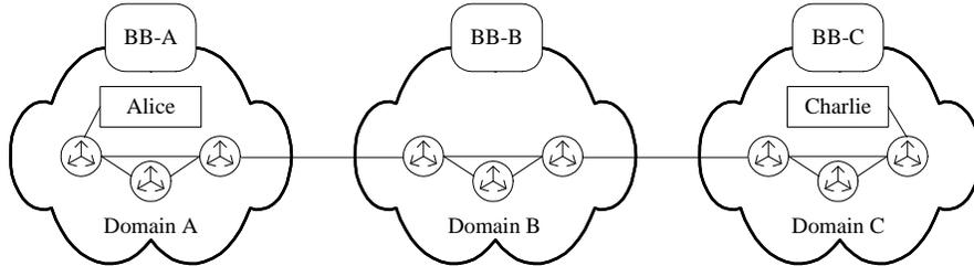
Figure 12. The multi-domain reservation problem. Alice needs to contact three BBs to make a network reservation from her computer in domain A to Charlie’s computer in domain C.
