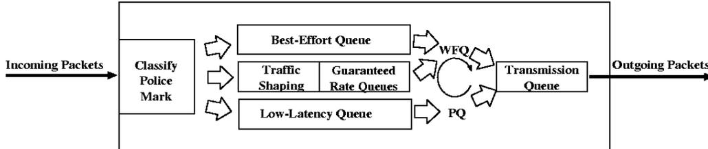
Figure 3. The ingress router configuration consists of a classification, policing and marking unit and of an optional traffic shaper. Traffic shaping is not applied for services that require a low latency, whereas guaranteed rate streams are shaped by applying a number of per-flow holding queues prior to WFQ scheduling.
