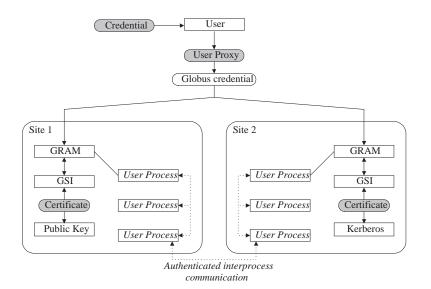
Figure 5: The Globus security infrastructure, showing its support for single sign-on and local heterogeneity
