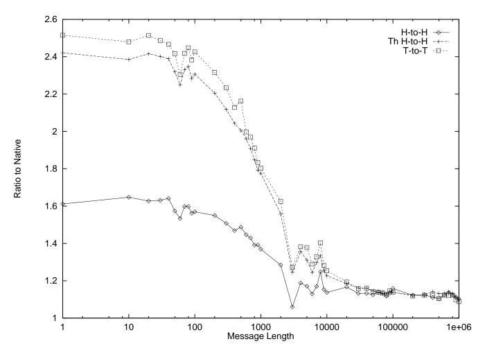
Figure 4: One-way message latency on the Sparc as a function of message size, relative to latencies achieved using low-level protocols, for three different cases, explained in the text: non-threaded handler-to-handler, threaded handler-to-threaded handler, and thread-to-thread.
